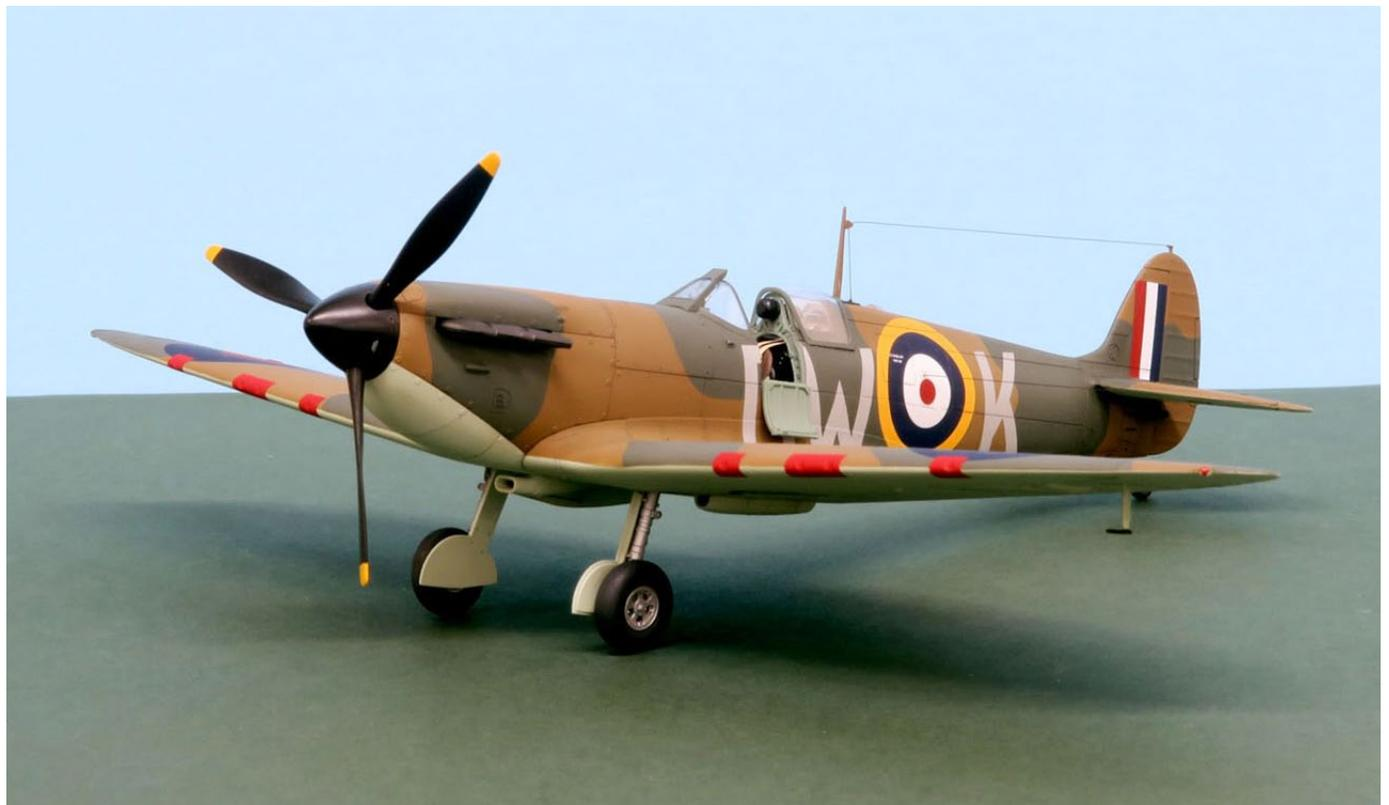
Here's Richard Price's eyecatching build of the brilliant new 1:48 scale Spitfire Mk. I from Tamiya. Richard assembled the kit OOB and painted it with Model Master enamels. Panel lines were accentuated with an AK Interactive wash. Decals are from the kit. Markings are for P9495 DW-K of RAF No 610 Squadron during the Battle of Britain, mid-1940.
